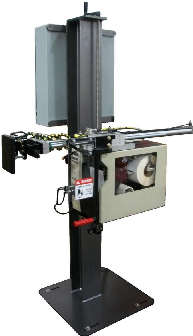
The Kolinahr Systems SA100 Automatic Pallet Labeler utilizes a desktop printer to print and apply labels to the side of a pallet load.
