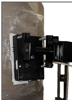
**Dual Label Operation** The label is applied to the leading edge when the pallet load pushes into the spring loaded tamp pad and moves the arm off of a proximity switch. The conveyor stops while the applicator arm returns to accept a duplicate label which is then wiped onto the side panel as the pallet load moves past the labeler.
